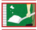
Step 4 - Cover entire area of Prograss using a ballast layer of clean sand and/or granulated rubber allowing extra around the edges and in the corners.
